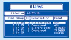
All alarm events are listed with timestamp and description. Pending alarms are indicated by a bell icon on the main screen and can be confirmed via the builtin keyboard.
