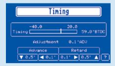
The MIC850 HMI module allows justification of various ignition parameters such as ignition timing and energy.
