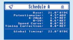
Overview of the ignition timing adjustment of configuration A. Here you can directly see whether ignition timing adjustment takes place via an analog input or via speed curve. The current ignition timing will be displayed under "Global Timing".
