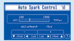
Display and adjustment options of the requested spark plug firing duration directly at the HMI-module.
