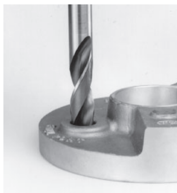
1. Drill a hole with a standard drill (see table)
